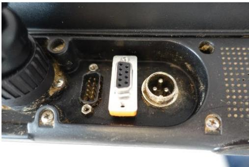
This way, the DB9 male connector of the connector can plug into the scale DB9 port originally female type.
