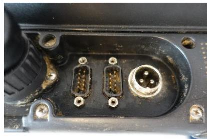
Note : On some scale heads such as the TruTest Eziweigh 7, one will need the TruTest DB9 adaptor cable as the connector on the back of the scale head is a proprietary round connector.
